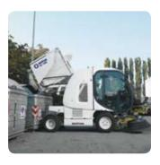
The multi-level dumping system enables emptying of the 1300 litre capacity hopper at heights from 80 to 160 cm
